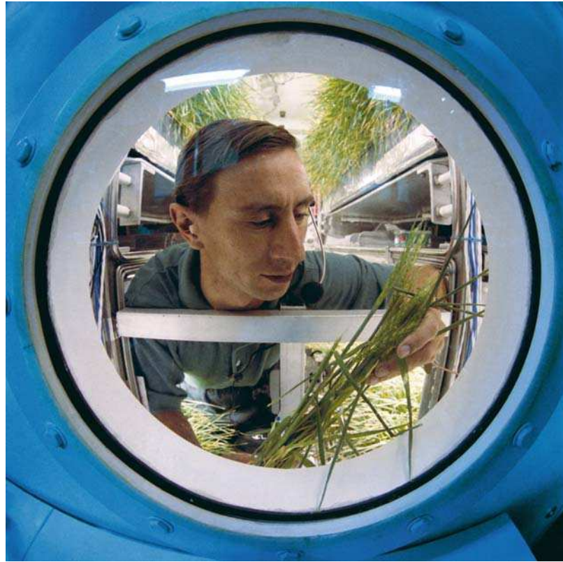
FIGURE 5.3 Test subject Nigel Packam inside a sealed chamber that used wheat to produce his oxygen (NASA photograph).
